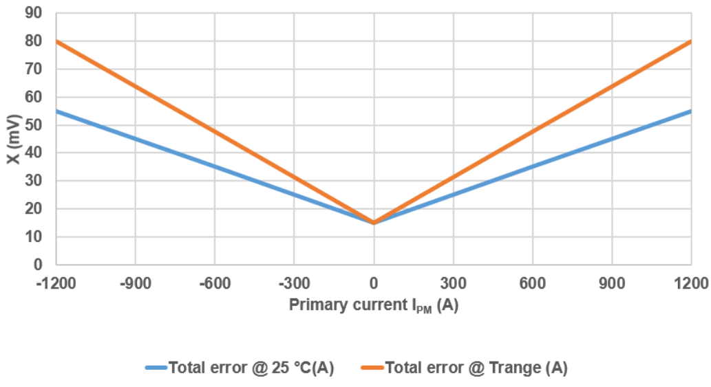
SHK-VBS-A3-S3: Overall accuracy X @ V_{CC} 5V (-40^{\circ}C \leq T_a \leq 125^{\circ}C) absolute error
