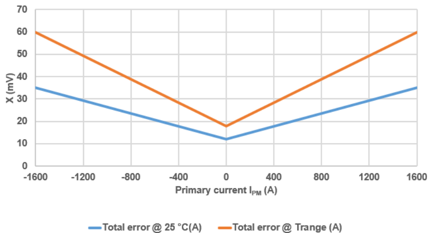
SHK-VBS3-SA/SHK-VBS3-SC: Overall accuracy X @ Vcc 5V (-40°C ≤ Ta ≤ 125°C) absolute error
